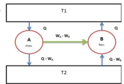
Hence it is concluded that reversible engine working between same temperature limits is more efficient than irreversible engine thereby proving Carnot's theorem.
