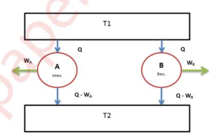
receive same quantity of heat Q from the source at temperature  $T_1.$  WA and  $W_B$  be the work output from the engines and their corresponding heat rejections be  $(Q-W_A)$  and  $(Q-W_B)$  respectively. Assume that the efficiency of the irreversible engine be more than the reversible engine i.e.  $\eta_A > \eta_B$  Hence,  $W_A Q > W_B Q$  i.e  $W_A > W_B$ .
