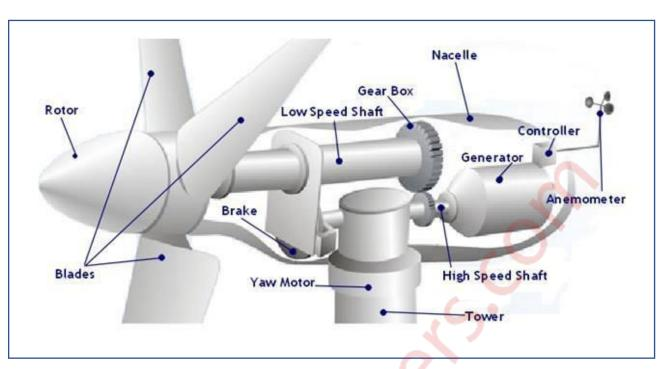
The schematic of the wind turbine components are shown here.
