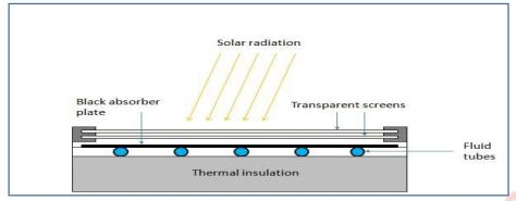
The schematic of a flat plate solar collector with liquid transport medium is given here.
