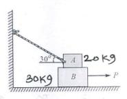
b. For given system find resultant and its point of application with respect to point A. [6]
