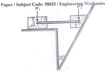
b. For the system shown in fig. if the collar is moving upwards with a velocity [8] of 1.5m/s. Locate the ICR for the instant shown. Determine angular velocity of rod AB, Velocity of A and velocity at the midpoint of AB.
