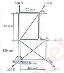
c. The resultant of the three concurrent space forces at A is R= - 788j N. Find [4] magnitude of F<sub>1</sub>, F<sub>2</sub>, F<sub>3</sub> forces.
