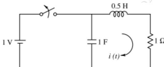
Switch is opened at  $t=0$ , steady state condition is reached before  $t=0$ . Find  $i(t)$  using laplace transform.
