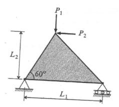
Data:  $L_1 = 0.6 \text{ m}$   $L_2 = 0.4 \text{ m}$   $P_1 = 5 \text{ kN}$   $P_2 = 2 \text{ kN}$  E = 180 GPa  $A = 6 \text{ cm}^2 \text{ for all}$ elements
