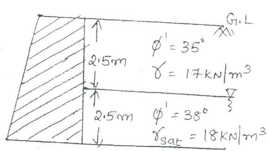
Q.4 a. A rectangular footing 2x3m rests on soil with its base at 1.5m below ground surface. calculate the safe bearing capacity using the factor of safety 3 on 08
