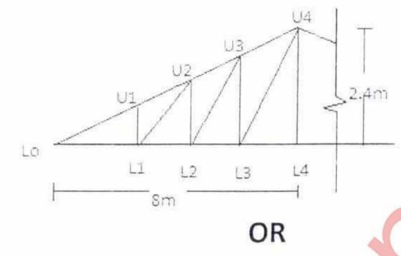
The flooring system of an industrial shed is planned as shown in fig Design Beam SB1 And MB1 And a beam to beam connection between them with top flange of beam at same level . Use ISMB section to design beam assuming beam to be laterally supported throughout. For following data
