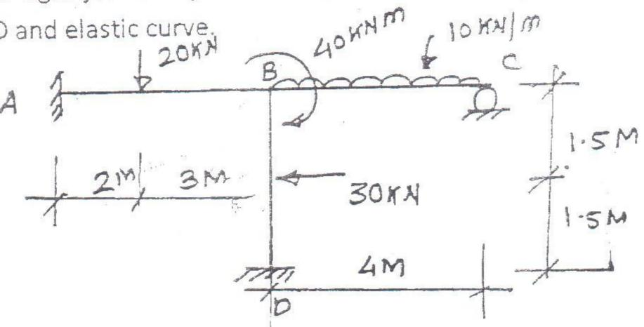
b) Analyse the beam by three moment theorem and draw BMD
