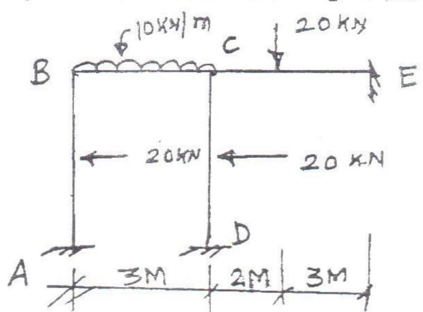
b) Calculate the plastic moment capacity required for the continuous beam with working load
