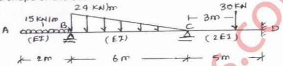
A rigid jointed plane frame loaded as shown in figure. Analyse this frame (16) using Stiffness method OR Slope-deflection method. Also draw BMD and deflected shape of the frame.
