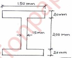
b) Find the plastic moment capacity 'M<sub>p</sub>' for the continuous beam shown in figure below. (08)
