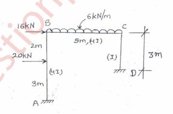
Q4). Using Stiffness matrix method, analyse the given portal frame. Draw BMD and deflected (20) shape.
