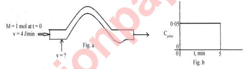
Q.2.b) The data given below represent a continuous response to a pulse input into a closed vessel which is to be used as a chemical reactor. Calculate the mean residence time of fluid in the vessel. Tabulate and construct the E curve.
