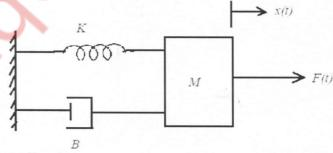
Find i) Transfer function, ii) Damping factor, ii) Natural frequency, iii) Percent overshoot, iv) Peak time, Assume: K = 33 N/m, B = 15 N-s/m, M = 35 kg
