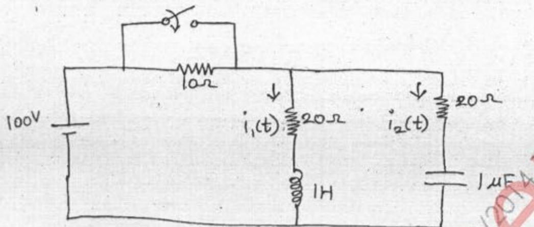
3. (a) For the network shown, write down tie-set matrix and obtain the network 10 equilibrium equation in matrix form using KVL. Calculate loop currents.
