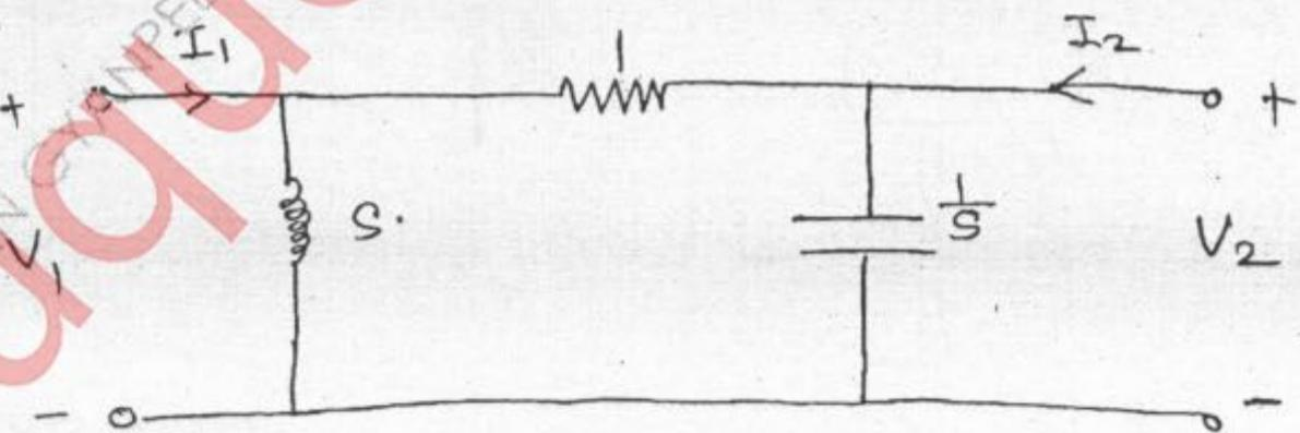
4. (a) Determine voltages  $V_1$  and  $V_2$  using superposition theorem.
