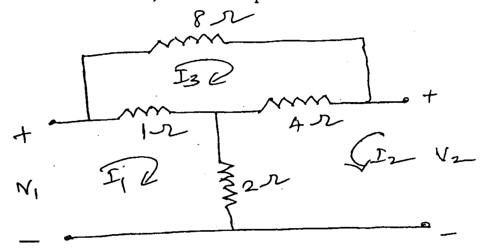
(b) Derive condition for recipro city in terms of Z parameters and symmetry in terms of h parameters.
