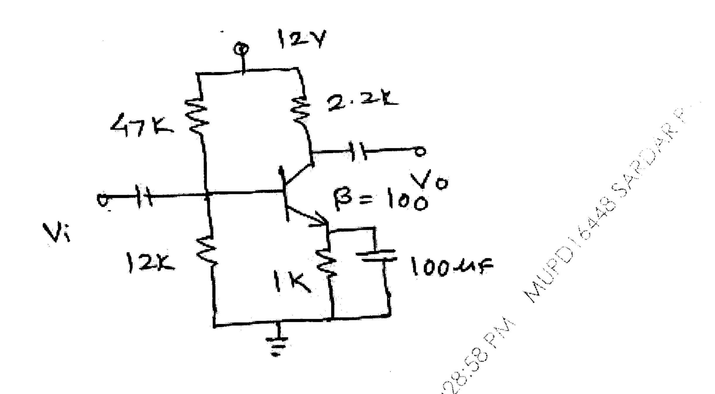
(b) Determine  $A_v$ ,  $Z_i$  and  $Z_o$  for the following circuit.
