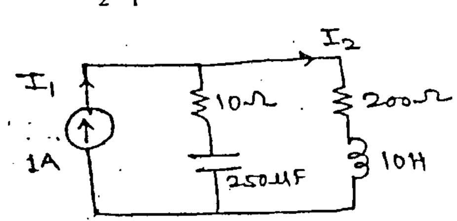
6. (a) Two identical sections of the network shown are connected in cascade manner. Obtain the transmission line parameters of over all connection.
