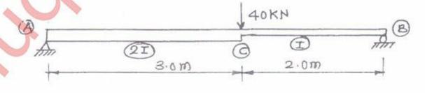
(a) Using Macaulay's method, determine maximum deflection and slope at the 06 supports. Take EI = Constant.
