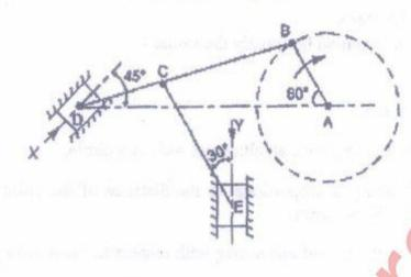
The crank AB turns uniformly at 180 rpm in the clockwise direction and the blocks at D and E are working in frictionless guides. Draw the velocity diagram for the mechanism and find the velocities of the sliders D and E in their guides.
