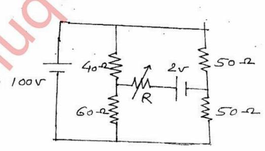
(b) Calculate the branch current I, and I2 for the circuit shown in Figure.
