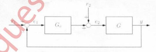
Determine the internal stability if  $G = \frac{1}{z-1}$  and  $G_C = \frac{1.5z-1}{z-1}$ .
